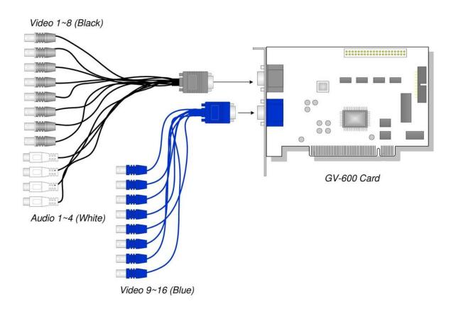
Figure 1-4 D-type GV-600 Card connections
